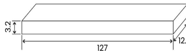
Dimensions of 3- Point Bending Specimen (Unit: mm)
